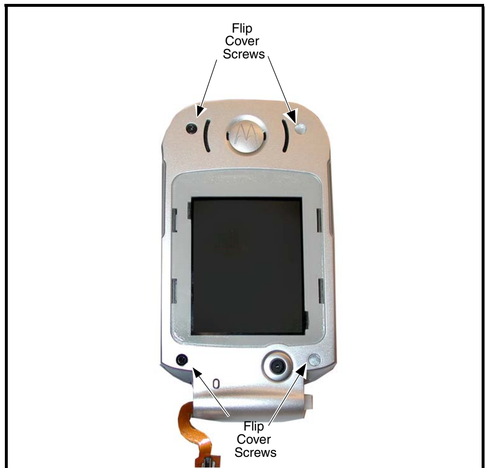
Figure 16. Removing the Flip Cover Screws
