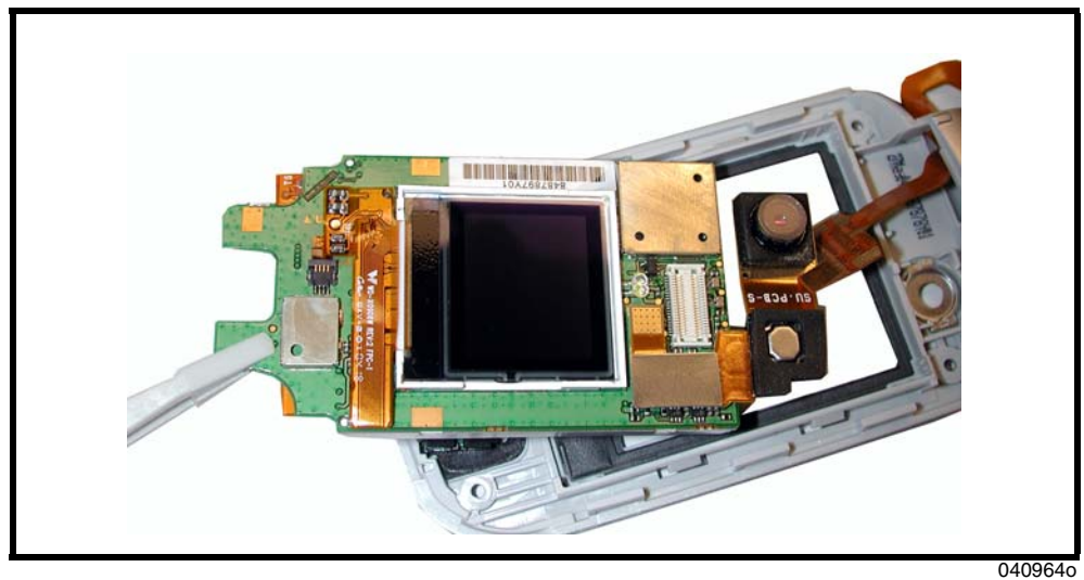
Figure 21. Removing the Display Assembly
